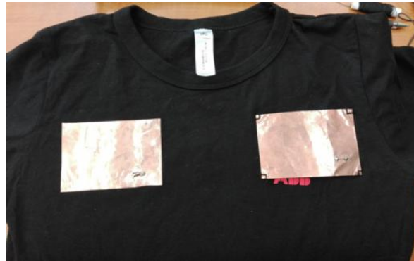
Fig. 7. Proposed portable and contactless ECG T-shirt
