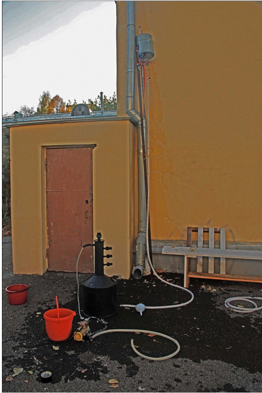
Fig. 2. The bottom nozzle of the tank is connected by a silicon pipe with the upper reservoir
