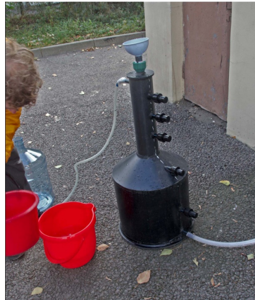
Fig. 1. Plastic tank with nozzles. Water is poured by the top orifice. Through the top nozzle an air from the pump is coming in. The lower nozzle where water comes out is attached to the silicon pipe. All other nozzles are plugged
