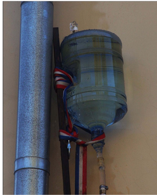
Fig. 3. Water fills the upper reservoir and poured from it with low speed corresponding to the speed of air supply to the lower tank
