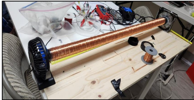
Fig. 2. Picture of coil-wound wave energy generator bars
