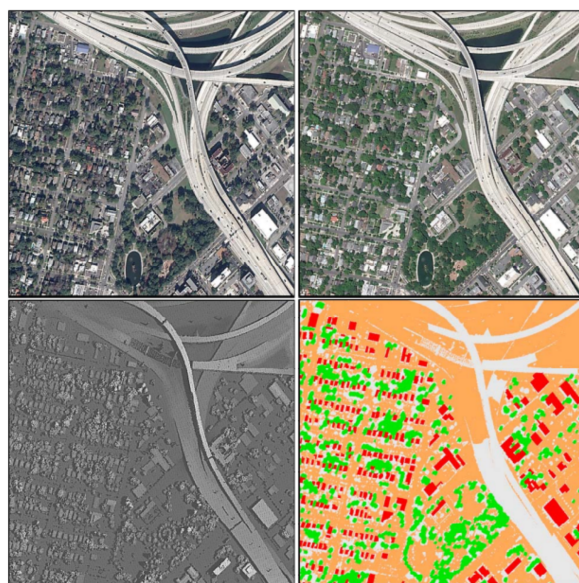
Figure 18. Examples from the US3D dataset. Epipolar rectified images (top) with ground truth left disparities and semantic labels (bottom).
