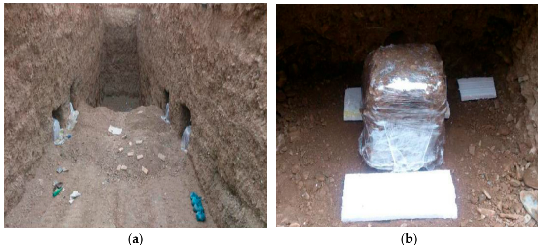
Figure 3. In situ direct shear strength test: (a) an access trench, (b) an intact cubic soil sample.
