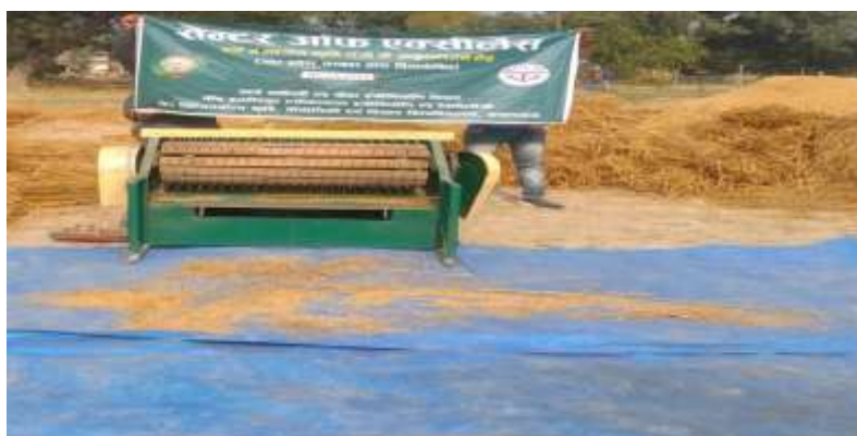
Fig. 6. Developed pedal cum power operated hybrid thresher
