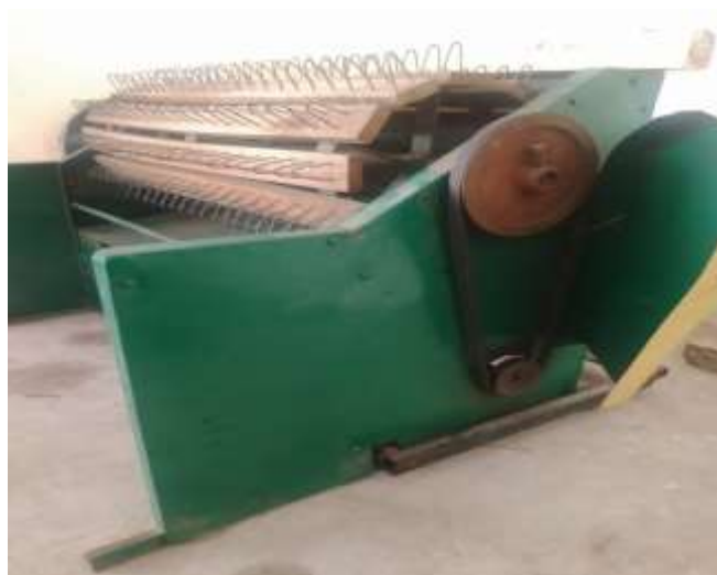
Fig. (5). Right side and left side view of pedal cum power operated hybrid thresher (case- 2)
