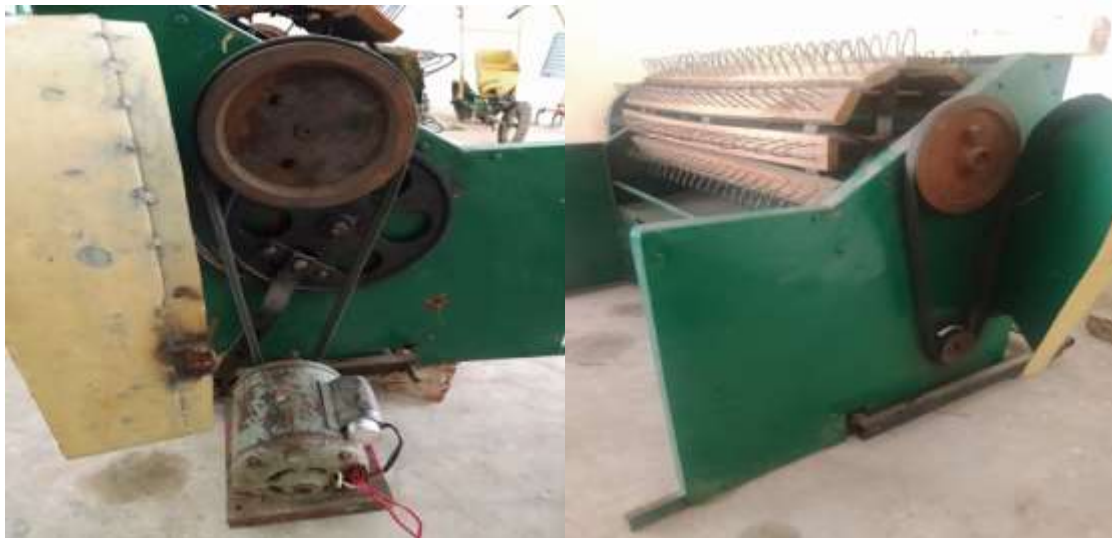
Fig. (3). Right side and left side view of pedal cum power operated hybrid thresher (Case-1)
