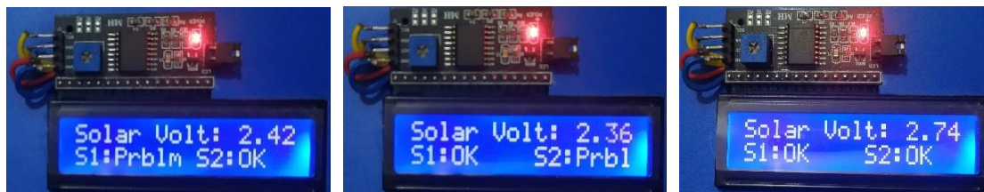
Fig. 10. Generated voltage and branch connection statuses on the LCD screen
