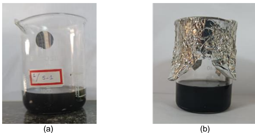
Fig. 2. Samples in solvent (a) o-Xylene & (b) Toluene after treating for 1 hour at 80°C
