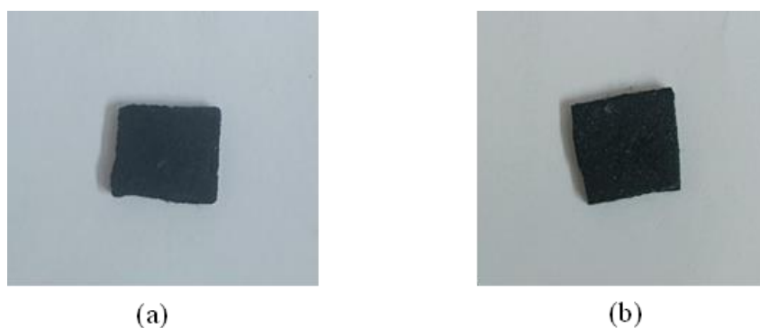
Fig. 2. Samples in solvent (a) o-Xylene & (b) Toluene after treating for 1 hour at 80°C
