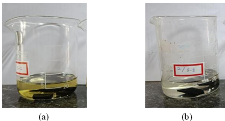
Fig. 1. Addition of solvent (a) o-Xylene & (b) Toluene and BPO to the reclaimed rubber
