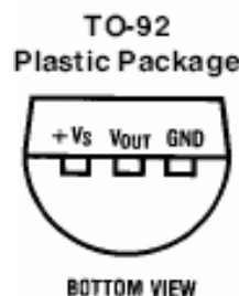
Fig. 1. Bottom view of LM35 temperature sensor showing pin out
